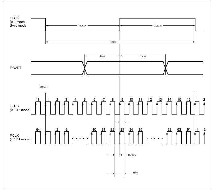
• SYBRK Signal Timing for External Synchronous mode
